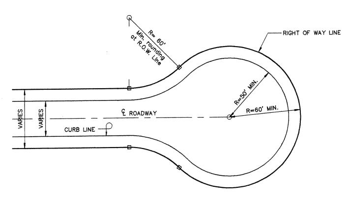
NOTE: THE CUL-DE-SACS SHOWN ARE ONLY TWO MINIMUM ARRANGEMENTS OUT OF MANY POSSIBILITIES. CUL-DE-SACS SHALL BE DESIGNED SO AS TO PROPERLY HANDLE THE TYPE AND AMOUNT OF TRAFFIC INVOLVED.
