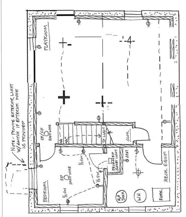
NOTE - ADD BATTERY POWERED SMOKE & CO DETENTORS IN LOCATIONS REO'D, BY CODE THROUGHOUT HOUSE WHERE NONE EXIST.
